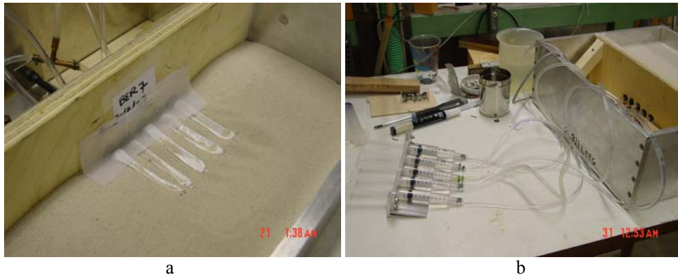
Fig. 2 Test setup for simulating expanding tubes in the centrifuge; a) installing empty tubes; b) syringe system for expanding tubes.
